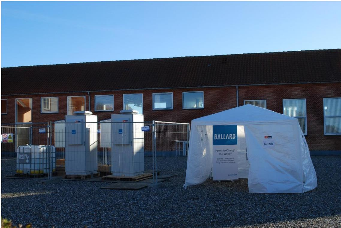
During the FAT Factory acceptance test the fuel consumption has been verified based on the systems internal fuel gauge and the tank size being 75L. According to the datasheet the fuel consumption is 1,4L/kWh. And therefore, it is possible to operate the system for 2 full days at 2kW load without refueling. The fuel level reads 37% and it took ~11,5h. to empty the tank. The produced electricity corresponds to ~23kWh. Table with the result:
