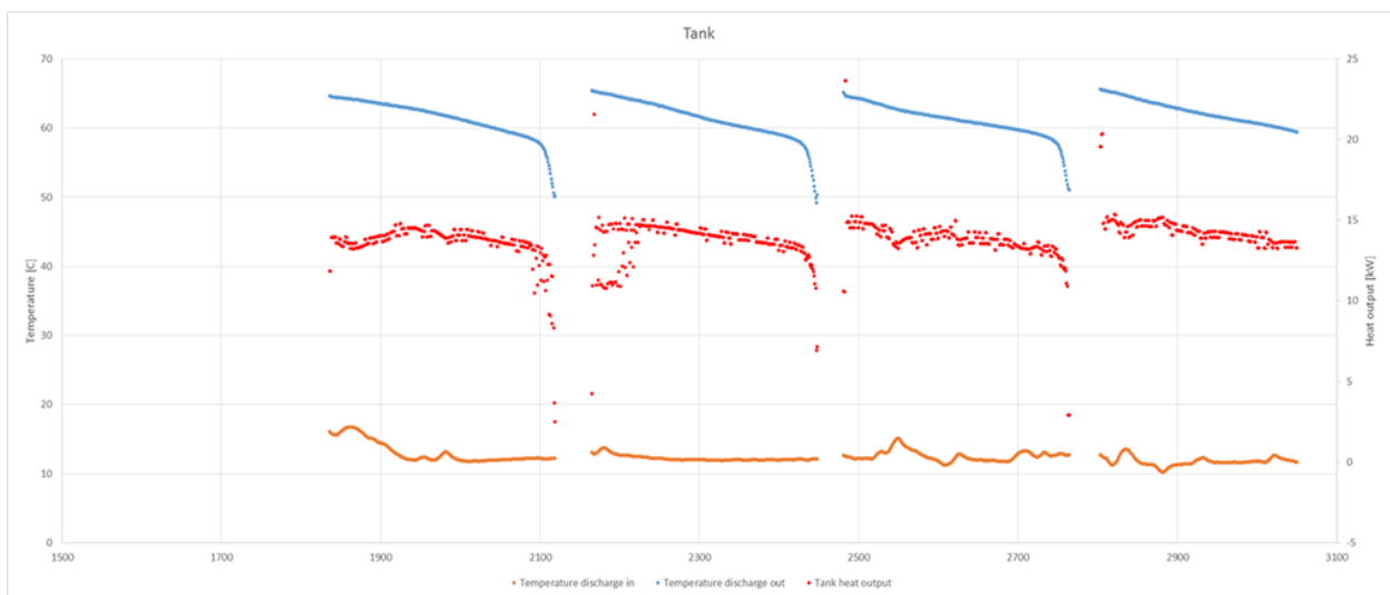
Figure 33 - The inlet (orange) and outlet (blue) temperatures (°C) during discharge and the output capacity (kW) from the storage tank (red curve).
