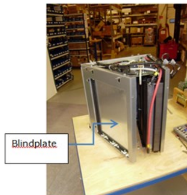
Figure 7 2,5kW scalable system consists of one 66cell stack compared with 2 stacks in an 5kW system. Blind plate is mounted Instead of the missing stack in order to keep airflow intact.
