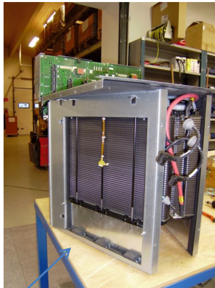
Figure 6 3,2kW scalable system mechanical components are unchanged compared with 5kW system. Blind plates are added on top of each cell stack to reach the height of a 66 cell stack.
