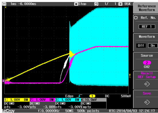
Figure 21 [The Yellow is the main supply voltages, the red is the supply voltages to the RS485 Driver and the Blue is D1. The white ref is driver supply voltages with 100nF bypass capacitor.]
