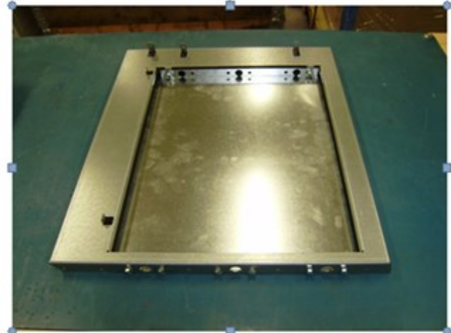
Figure 8 2,5kW scalable system in real. Blind plate that replace on 66cell stack is needed to be tight in order to keep airflow intact for the remaining 66cell stack
