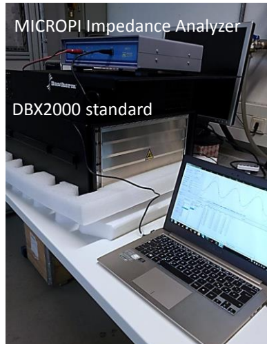
Figure 1.7 – DBX2000 standard system with external impedance analyser to measure the EIS spectra in switched-off conditions.
