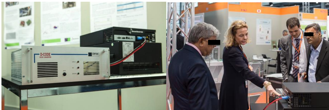
Figure 1.4.2 - DBX FCS connected to the HV DC/DC Converter on display at the Hannover Fair 2014 (left); Prof. Marie-Cécile Péra explains to visitors the equipment at the Hannover Fair 2014 booth (right).
