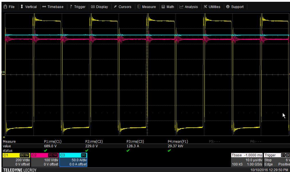
Fig. 5.18. Continuous operation testing of one phase of the DC/DC converter block (low power).
