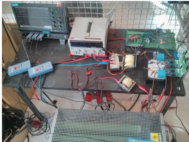
Fig. 5.14. Testing of a new DSP adapter board.
