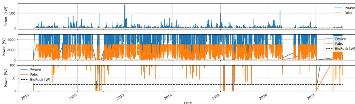
**Figure 6** – Wave Power in Hanstholm from 2015 to 2021 (blue). Expected power production of one 3kW Resenwaves device at location (orange). Power consumption of one induced mineral deposition installation made of rebar steel for a total of 50 kg.
