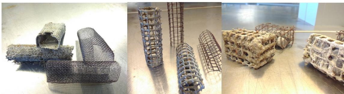
**Figure 2** - Cathodes electrified for 9 months and covered in mineral deposition, and cathodes not tested, first Hanstholm Installation.
