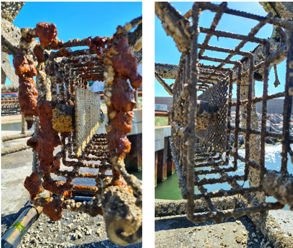
**Figure 3** – The two setups in Hanstholm, the cathode is the metal construction where the metal plate in the middle of the construction is the anode. (left) The setup disconnected from the power supply showing extensive corrosion. (right) Setup connected to power source with seashells and biofouling growing on the cathode and the PVC structure.
