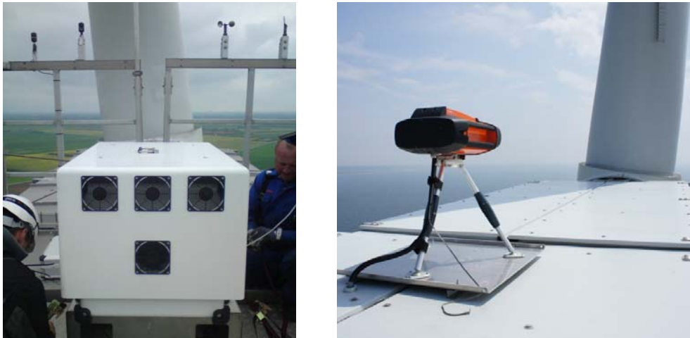
Figure 1 Prototype Leosphere nacelle lidar to the left, and production wind iris nacelle lidar from Avent Lidar Technology on the right
