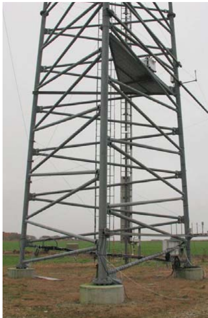
Figure 7 The 10m platform for mounting the nacelle lidar at the Høvsøre met mast to the left. The 10m mast with the top mounted sonic to the right. Met mast is shown in the background. The cross bar is used for identification of lidar beam position and is not used in calibration measurements.
