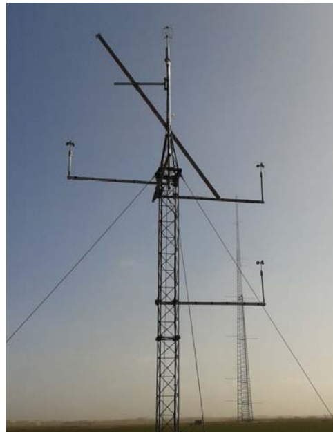
Figure 7 The 10m platform for mounting the nacelle lidar at the Høvsøre met mast to the left. The 10m mast with the top mounted sonic to the right. Met mast is shown in the background. The cross bar is used for identification of lidar beam position and is not used in calibration measurements.
