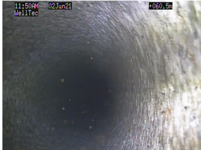
Above: Part of the 8 1/2" hammer-drilled borehole where the most upper packer was set at 60 meters.
