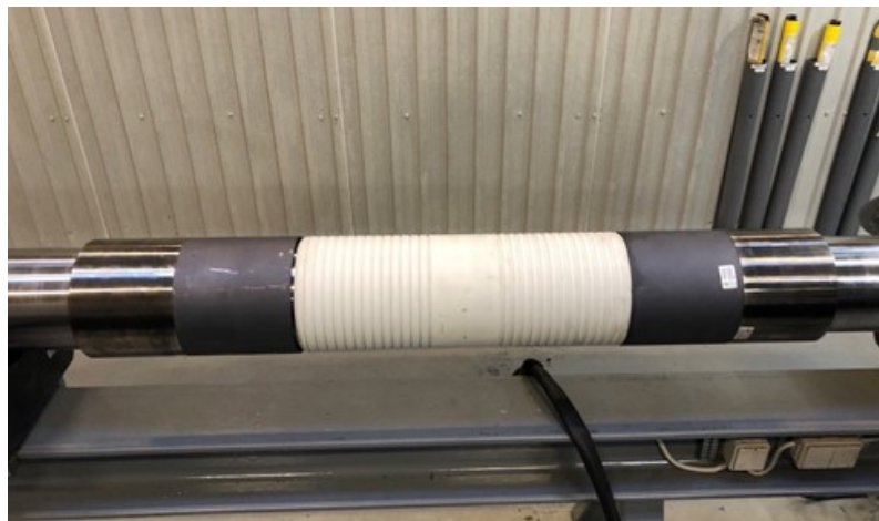
Above: The assembled new high expansion packer design being assembled and prepared for testing.
