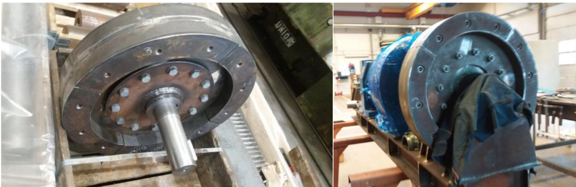
Figure 13. The flywheel currently installed on the Tordenskiold's PTO.
