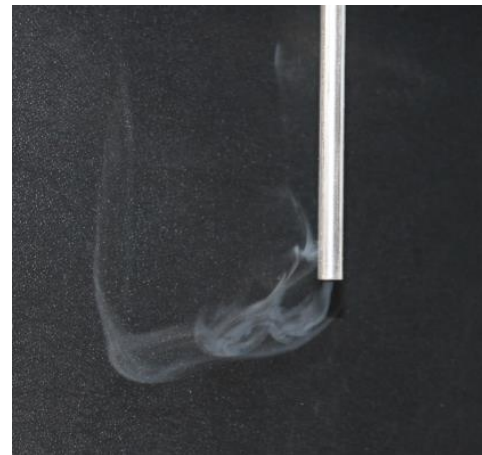
Fig. 5.11 a) Oxygen permeation flux of a 35 \text{ cm}^2 CGO-LSF membrane tested in the partial oxidation test unit adjacent to a LT-CFB gasifier at 850 \text{ }^\circ\text{C} . b) White producer gas at the output of the membrane indicating the partial oxidation of the tars.
