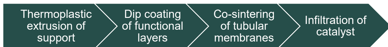
Figure 5.2. Major steps in the fabrication of tubular asymmetric OTM at DTU Energy.
