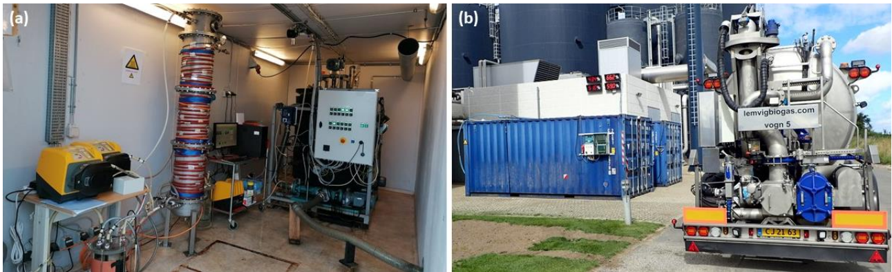
Fig. 13. Constructed prototype biogas upgrading unit and operational demonstration at Lemvig biogas plant
