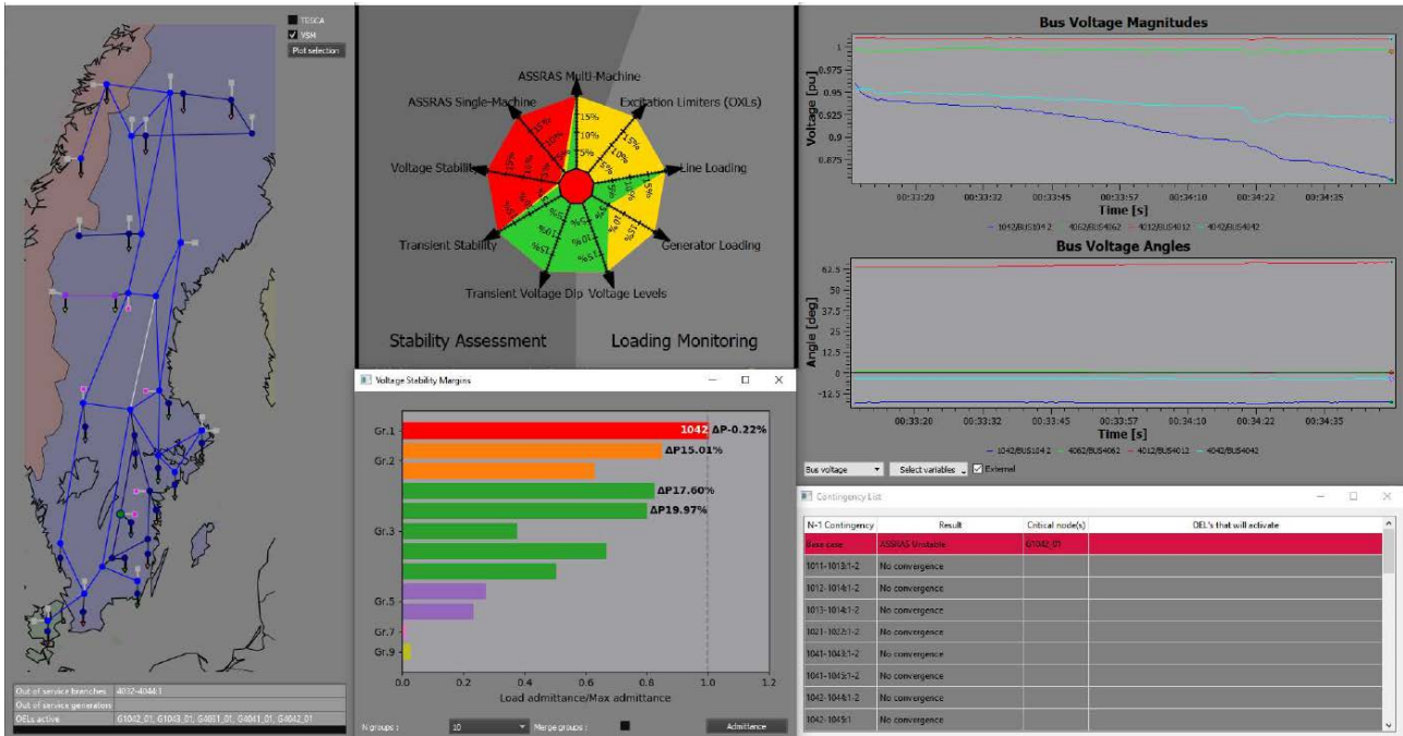
Figure 11: Snapshot from the demonstration (figure 10) at an instance of time where system instability had been identified by the real-time applications.
